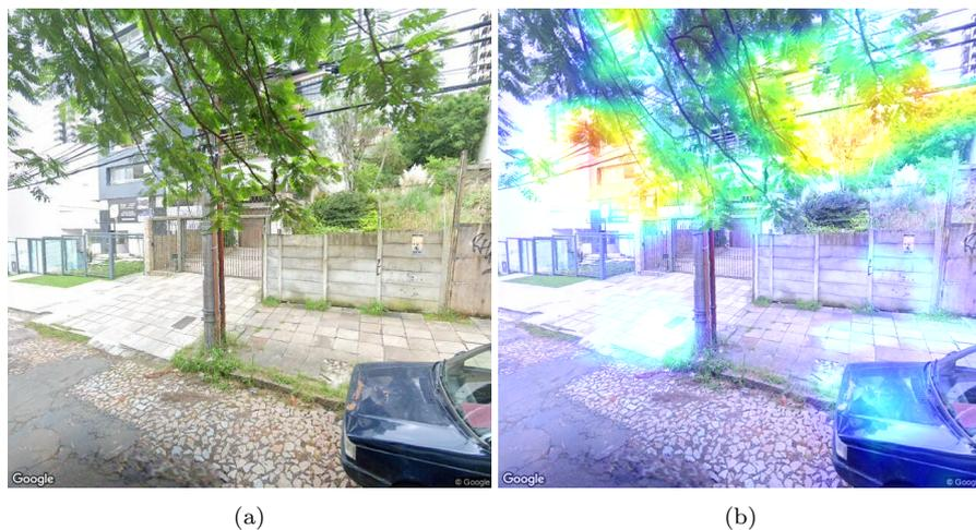
Fig. 11: (a): An image misclassified as having an entanglement between tree and electric wires. Due to the position of the camera just below the foliage it seems that indeed there is an entanglement, but directly using Google Street View to navigate to another position reveals that the entanglement does not occur. (b): The salience map generated with the Grad-CAM++ method reveals that the main relevant regions (in red) observed by the network were the branches and the wires in the image.
